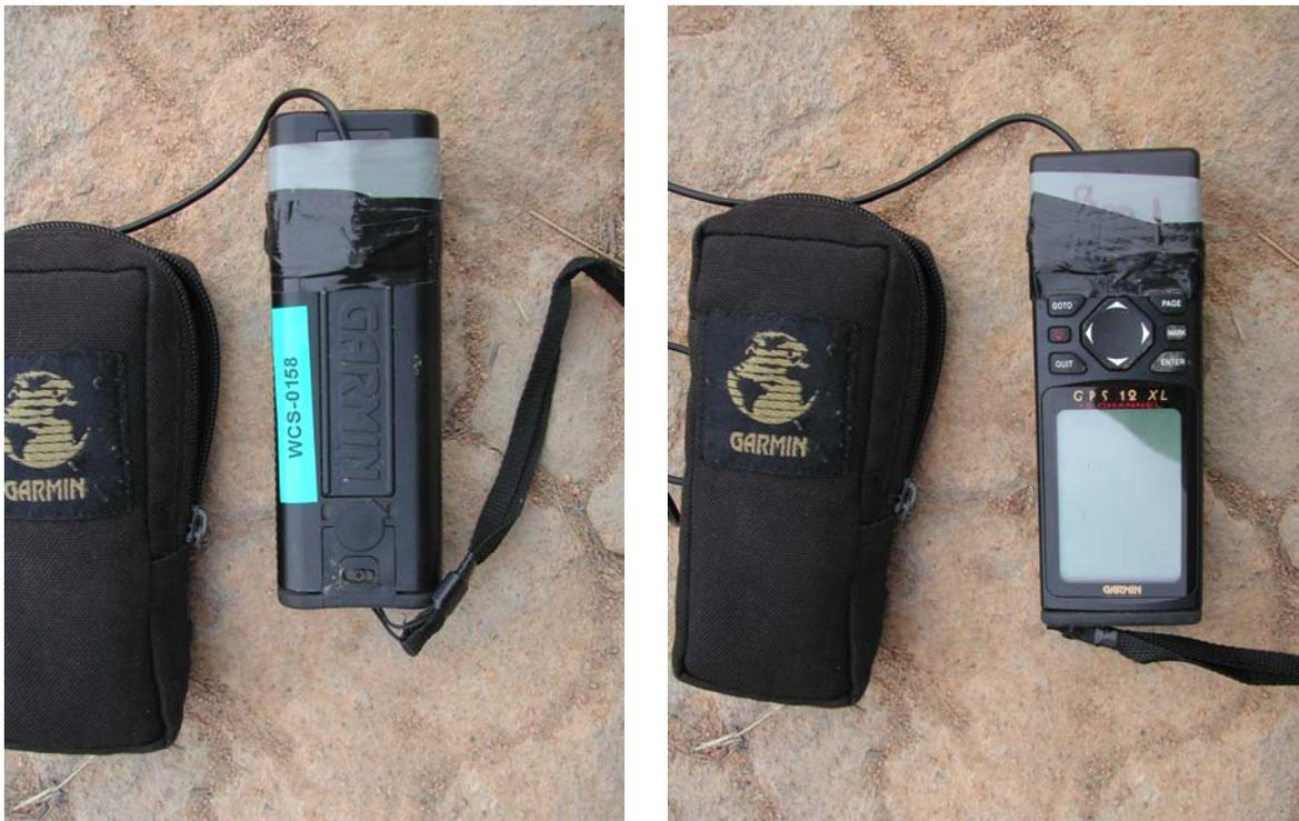
Some cheaper types of antenna are available which plug into the back of the GPS but which are easily broken off in forest conditions, where the user is moving all the time. These cheaper antennae are designed for use in a vehicle where the GPS is attached to an immovable surface, and should not be used in the bush: buy the ones where the cable sits flush with the back of the GPS unit (Fig 6).
