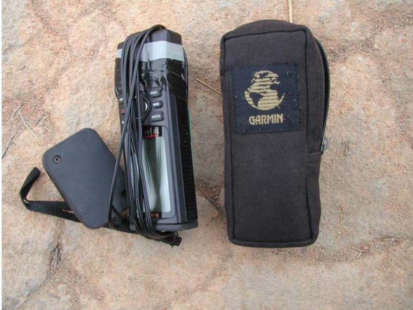
Fig. 9. Correct storage of antenna and GPS unit.
